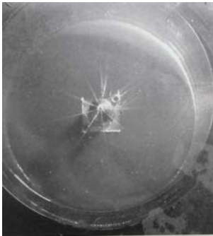
Injector spray pattern without FUEL PREPARATOR
