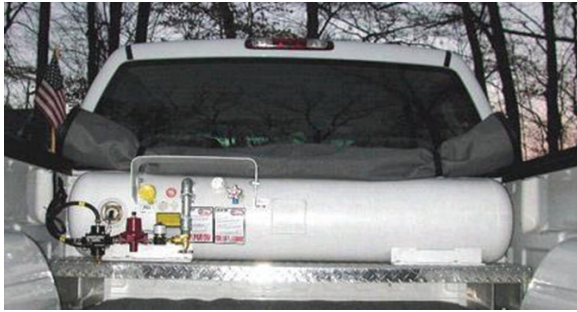
Pickup bed propane tank installation.
