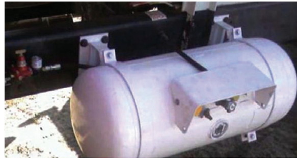
Large truck frame propane tank installation.
