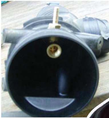
Propane injection nozzle
